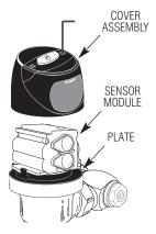
Install Battery Compartment Cover and secure with Retaining Screw. Make certain that Battery Compartment Cover is fully compressed against Gasket to provide a seal; **Do Not** overtighten. Plug the Electrical Connector into the Battery Compartment Cover. Reinstall the Sensor Module onto the Plate. Reinstall the complete Cover Assembly onto the Plate. Tighten the two (2) Screws on top of the unit.
