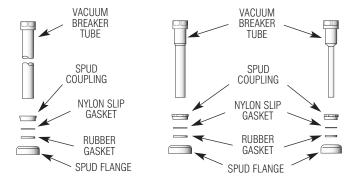
Insert Tube into Fixture Spud.
