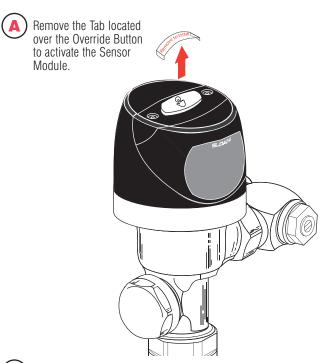
For the first ten (10) minutes of operation, a Visible Red Light flashes in the Sensing Window of the Optima *Plus* Flushometer when a user is detected.
