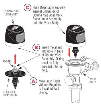
To facilitate installation, the O-ring on the diaphragm assembly must be wet for easier insertion.
