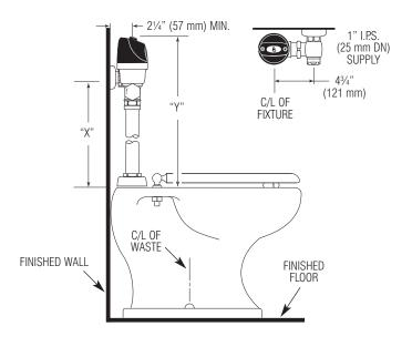
Model 8115 & 8116 valves are designed for installations where the water supply is roughed-in 24" - 27" (610 mm - 686 mm) above the top of the water closet.
